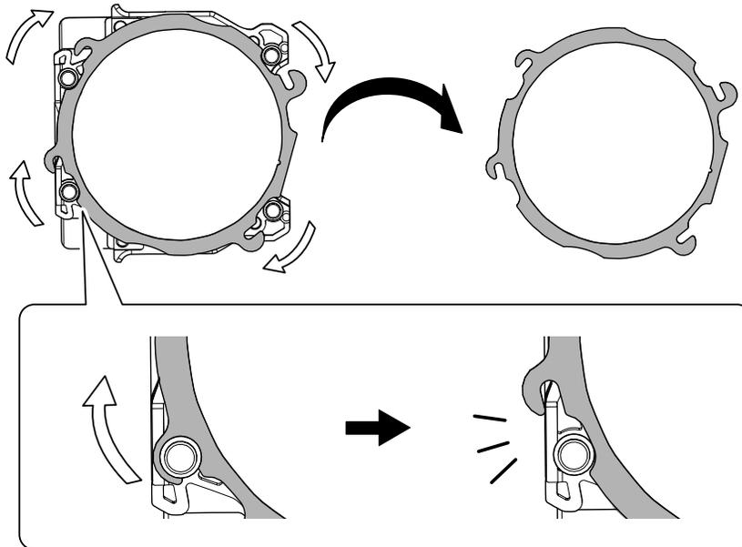
**3 Mount the pin-type workpiece adapter on the adapter base.**
