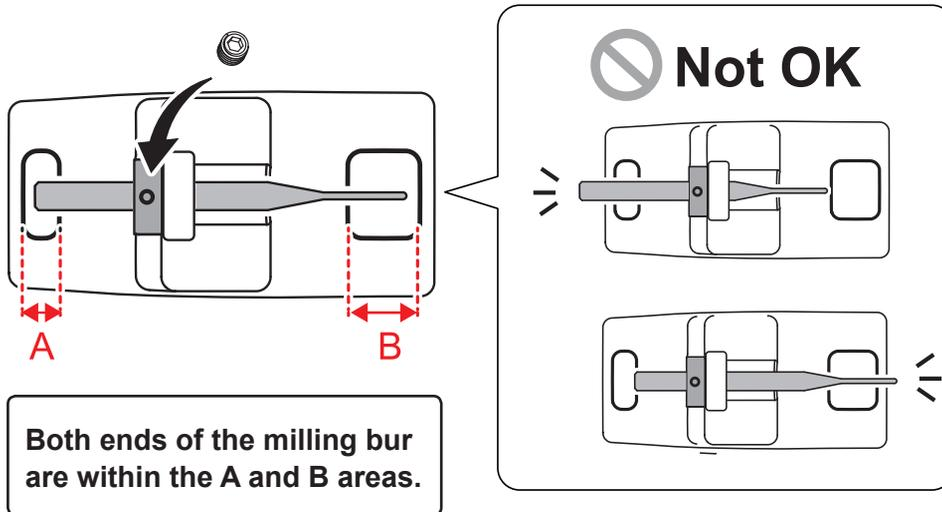
② Set the milling bur in the ATC magazine.
