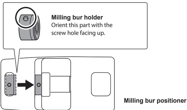
② Slide the milling bur through the milling bur holder, and determine the proper position.
