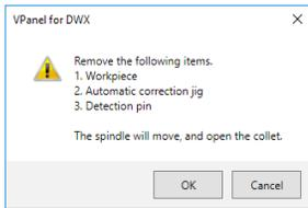
When the screen shown in the image on the left is displayed, click [OK]. The spindle unit will move, which will open the collet.
