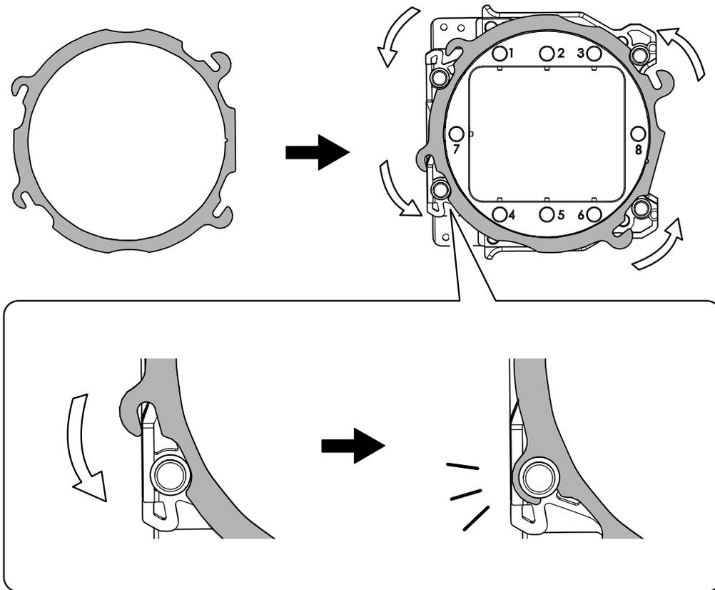
⑤ Use a torque screwdriver to tighten the screws in the positions shown in the figure. (4 locations)
