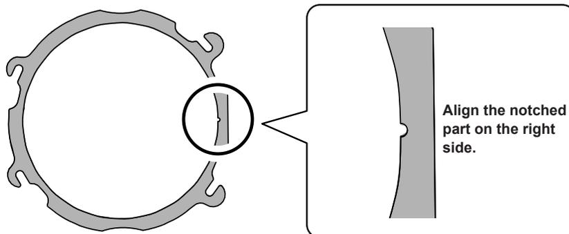
② Turn the adapter cap in the direction indicated by the arrows to attach it to the screws.
