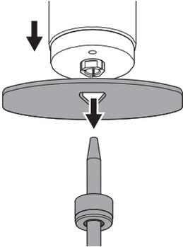
④ Remove the detection pin and the wrench.
