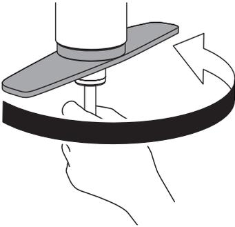
③ Tighten the collet with the wrench while holding the detection pin.
