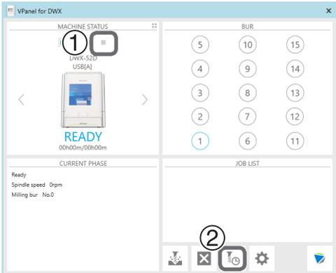
**1** In the top window of VPanel, select the machine for which you want to set Intelligent Tool Control.
